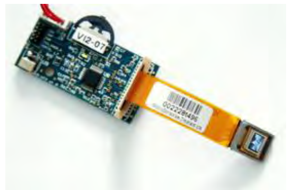
MED's tiny eyescreen microdisplay with a 6mm (0.24-inch) diagonal pixel array can be combined with magnifying optics to produce a large virtual image, that appears to the eye to be equivalent in dimensions to the picture on a TV screen or computer display.
