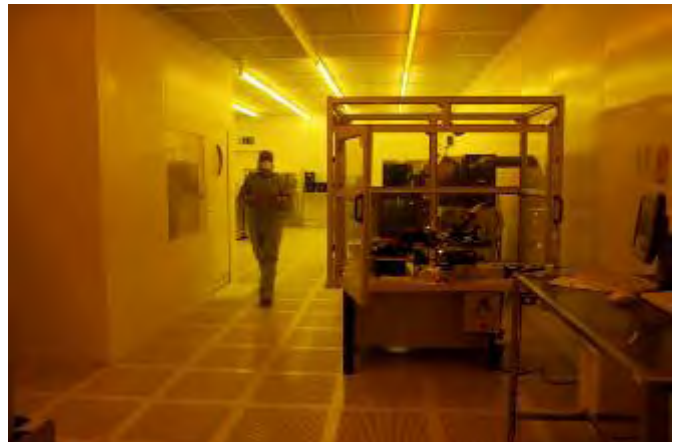
Although ForthDD does not produce its own silicon wafers, their facility in Dalgety Bay, Scotland does all the processing (coating, laminate assembly, cell filling, mounting, etc), providing advantages related to quality and scheduling.
