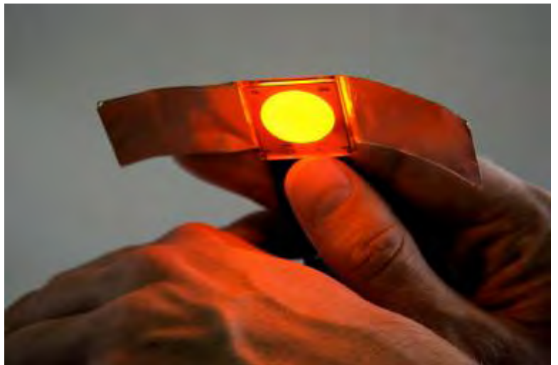
The OLED is packaged in a band-aid-like structure and applied directly to a skin cancer lesion.
