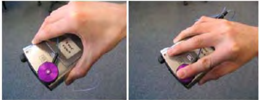
The vibro-tactile actuator on the back of an iPAQ
