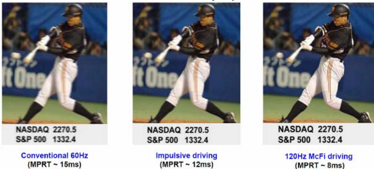
Figure 3: Result of Samsung's Method of using 120 Hz Frame-Rate with Interpolated-Motion Frames as a Means of Reducing Motion Blur
