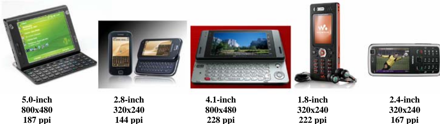
Figure 1: A selection of high-PPI mobile products -- presented by Barry Young from DisplaySearch
