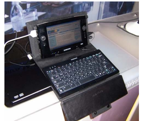
Figure 13: Samsung's UMPC in a "portfolio-style" case with an external keyboard and an external optical drive
